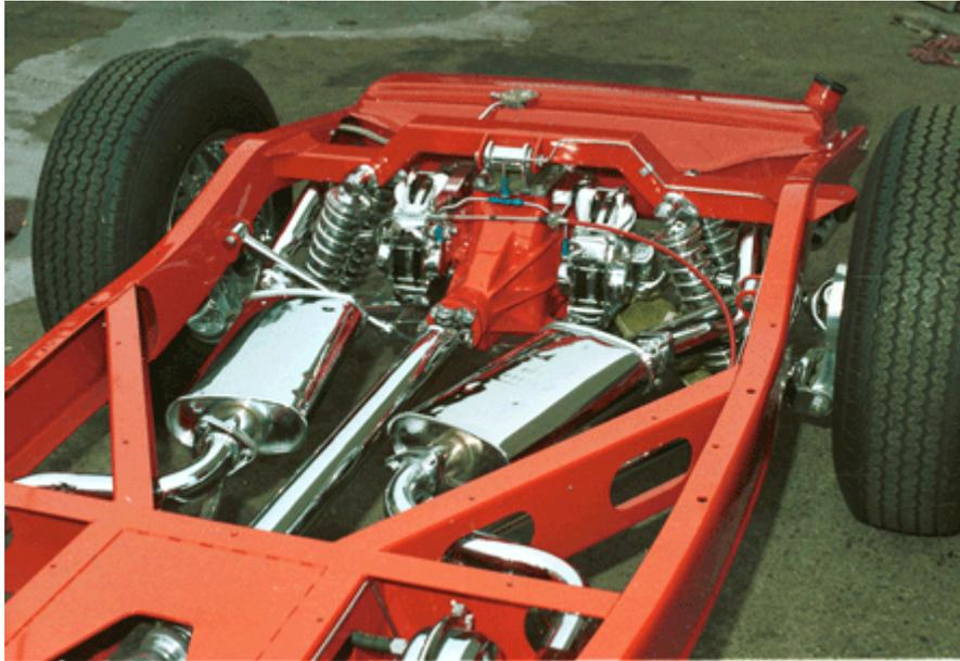
A good deal of common sense must be exercised in the assembly of this unit, high quality welds are essential, we recommend Heli-ARC (TIG) Welding. If you are in doubt about your welding ability, we strongly suggest that you tack weld components in place and take them to a competent or certified welder for final welding.
